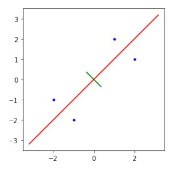
We see that the direction of maximum variance is given by the dominant eigenpair. The next eigenpair is **orthogonal**.
